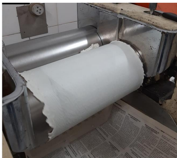
Figure 1: Illustration of the parallel roller mixer for sample production.
